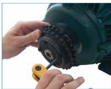
TIGHTEN SCREWS ALTERNATELY
