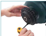
REMOVING A TAPER LOCK BUSH
