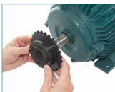
INSERT SCREWS AND LOCATE ON SHAFT
